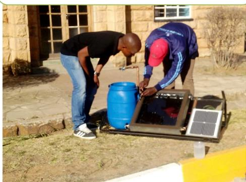
A solar water heating system using a solar-powered pump, mounted on the roof of a rural household for measurements, data logging, remote monitoring and analysis
